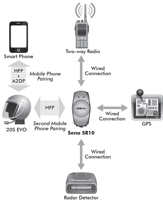
Parallel Connection of SR10 and Mobile Phone by Bluetooth Second Mobile Phone Pairing
